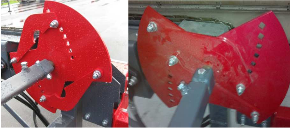
Figure 3. The in-feed disc adjusted for small and large logs
